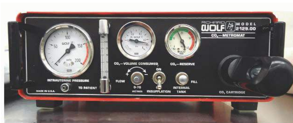
FIGURE 18.11 CO 2 is infused using a specific hysteroscopic insufflator that measures the flow rate (100 mL per minute) and uterine pressure (not to exceed 150 mm Hg). Laparoscopic CO 2 insufflation devices cannot be used for hysteroscopy due to a much higher flow rate designed to expand the abdominal cavity.
